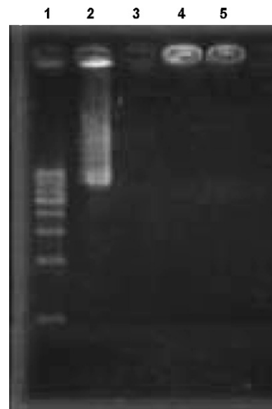
Fig. 3. Resistance of pDNA-PLGA/PEI nanosphere complex to DNase I degradation. Lane 1 is molecular weight marker. Lane 2 is naked pDNA. Lane 3 is digestion of naked pDNA with DNase I. Lane 4 is pDNA-PLGA/PEI nanosphere complexes. Lane 5 is digestion of pDNA-PLGA/PEI nanosphere complexes with DNase I.
